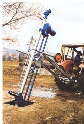
V-Pump with tractor lift attachment and winch assembly
