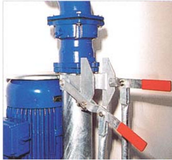
Handling lever for mixing and pumping
