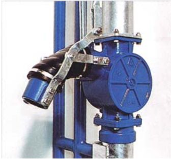
Mixing nozzle adjustable up (45°) and down (45°), therefore efficient destroying of floating crusts and sedimentations
